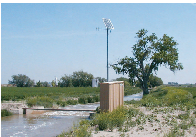
Figure 1. A rated canal section is remotely monitored using a SCADA system. RTU equipment is 12-volt DC powered from a solar panel that maintains a charge on a battery. Communication with the site is via radio
